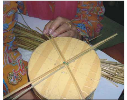
13. Starting a cylindrical box
